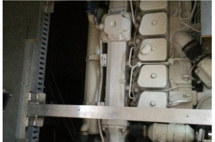
Starboard Cummins 6BTA 250hp diesel
