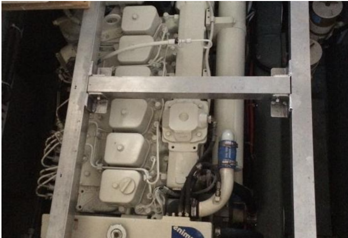
Port Cummins 6BTA 250hp diesel
