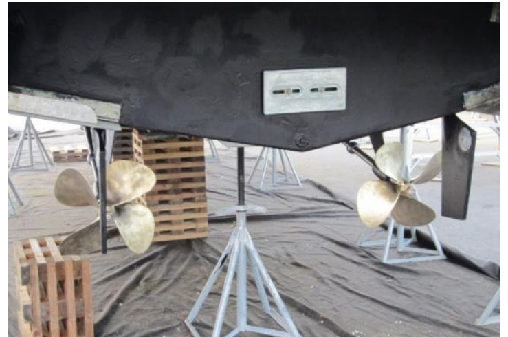
Props, cleaned, polished & zinc anodes replaced
