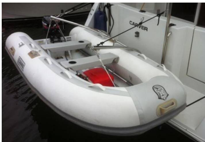
10' Titan RIB tender w/Mercury 15hp
