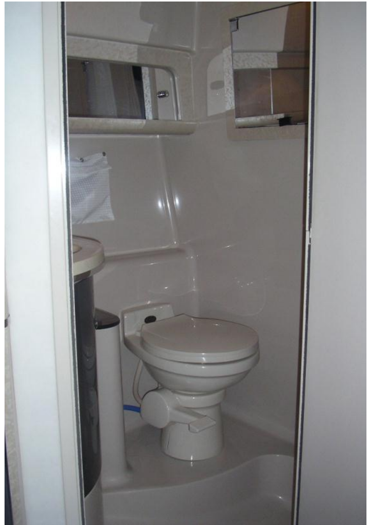
Head with VacuFlush system
